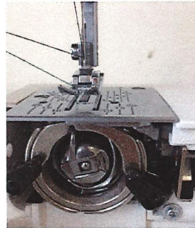
5. Pull the loop until you bring up the end of the thread.
