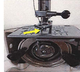
2. Keep winding the wheel towards you until the needle had gone down into the bobbin case.
