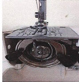
3. Keep winding the balance wheel towards you (keep hold of the top thread!) you will start to see the bobbin thread come up.
